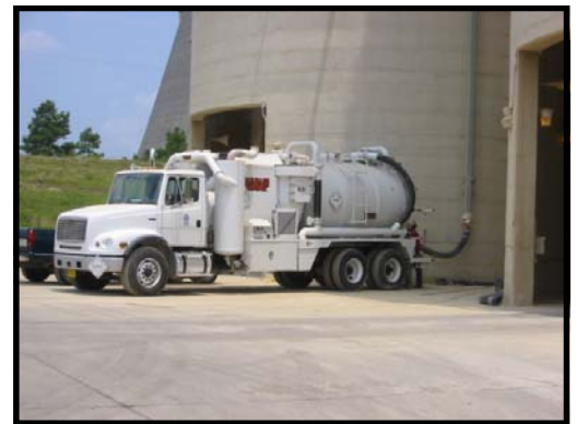
PMI Vacuum Truck removing fly ash at a electric generation plant in Arkansas.
